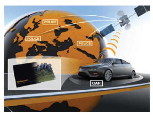
If the vehicle is stolen, the police or authorised service providers can monitor the vehicle on the screen and, if necessary, initiate a pursuit. Continental also offers the option of remote vehicle disabling. As soon as the vehicle is stopped for more than thirty seconds, Novanto acts to prevent the engine from being started again, putting an end to the thief's getaway.
