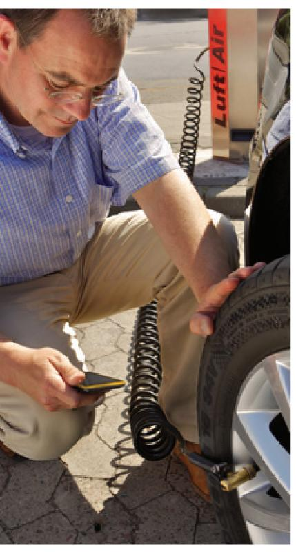
Continental's tire pressure monitoring system will soon be able to report to smart phones. The system also provides information about the correct pressure when tires are inflated. Enhanced driving safety and fuel efficiency are expected.
